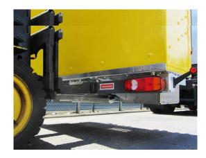
Disengage the bottom pins on both sides.
