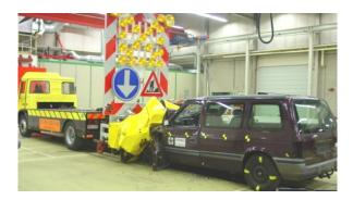
The truck-mounted crash attenuator (TMA) is a <u>mobile safety equipment</u> used during mobile or temporary road works in order to enhance protection to the work force against surrounding traffic hazards.
