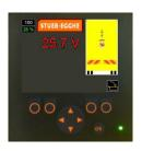
The movement of the cushion can be stopped at any moment with the button under the STOP icon.
