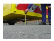
Should it be necessary to adjust the height of the cushion, raise the cushion (see Raising the cushion on p.13) and disconnect it (see Dismounting the equipment on p.15). Relocate the upper pins to the appropriate height.
