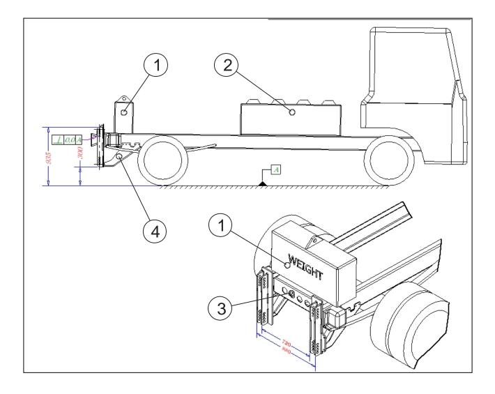
Make sure the truck is weighted to the desired mass before mounting the attachments.
