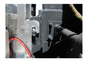
After engagement tilt the docking station as to align the holes at the bottom of the docking station and the frame
