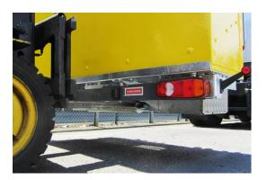
On the attachment frame insert the pins on both sides at the desired height
