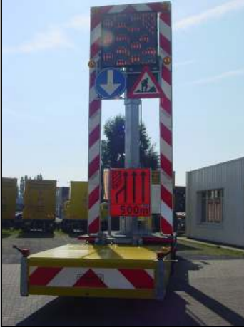
Variable messaging Sign Posting mounted on telescopic lift
